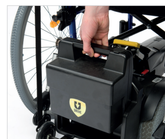
SIMPLE BATTERY REMOVAL
